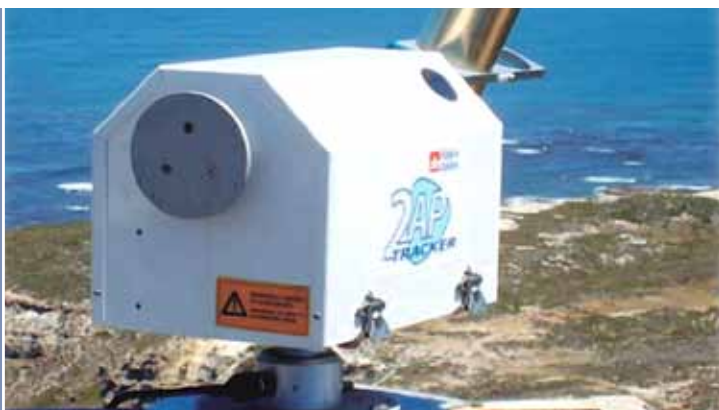
AP2 solar tracker measuring aerosol optical depth of the atmosphere
